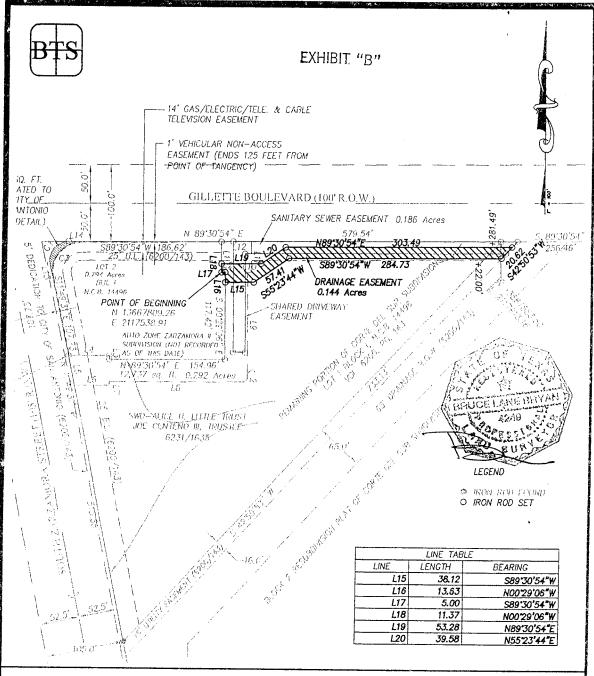
THIS IS TO CERTIFY THAT, ON THIS DATE, A TRUE AND ACCURATE SURVEY WAS MADE ON THE GROUND UNDER MY SUPERVISION OF PROPERTY SOUTHEAST OF THE INTERSECTION OF GILLETTE BOULEVARD AND ZARZAMORA STREET, IN BEXAR COUNTY, TEXAS, DESCRIBED AS FOLLOWS: A DRAINAGE EASEMENT OF VARYING WIDTH, BEING A 0.144 ACRE PORTION OF LAND, BEING MORE FULLY DESCRIBED IN THE FIELD NOTES ATTACHED HERETO AND MADE A PART HEREOF.
